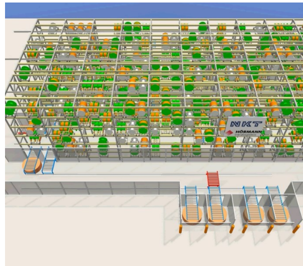
Illustration 2 Renewal of the conveyor technology at the automatic wire warehouse
