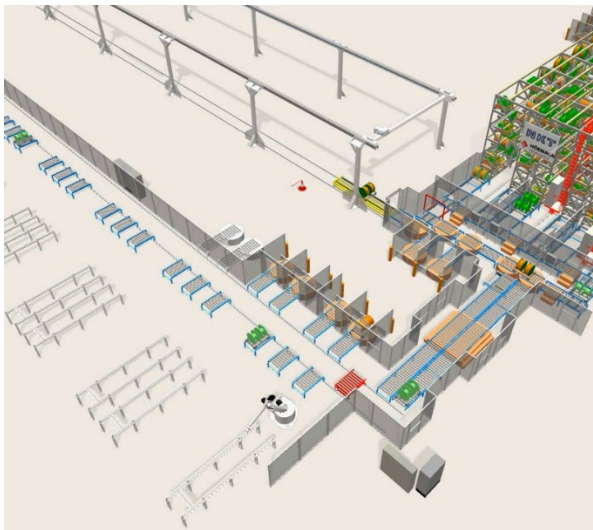
Illustration 1 Storage and retrieval stitch at the spool warehouse with automated connection to shipping and production
